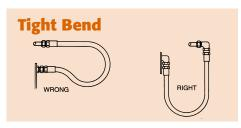
When radius is below the required minimum, use an angle adapter to avoid sharp bends.
