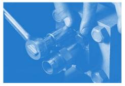
Lay the hose assembly into the routing position to verify length and correct routing.
